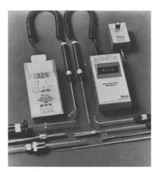
**POCKET-SIZED THERMOMETERS** Pocket-sized digital thermometer systems by Wahl Instruments, Inc. measure the temperature of surfaces, liquids, air and gases over a range of -100 to 550 C. The battery-operated Digital Heat-Prober LED model 392 and LCD model 350X mate with more than 20 2-point calibrated interchangeable low mass probes. The systems use platinum sensors for portable precision accuracy. Contact: Heat-Prober Division, Wahl Instruments, Inc., 5750 Hannum Ave., Culver City, CA 90230.
